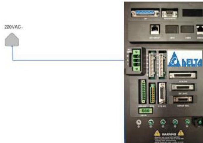
Figure 4-2 Power connection diagram of Python550F-D6
