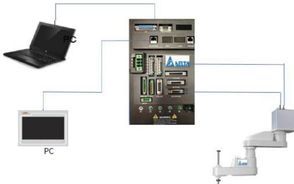
Figure 4-1 Typical system application wiring diagram of Python550F-D6
