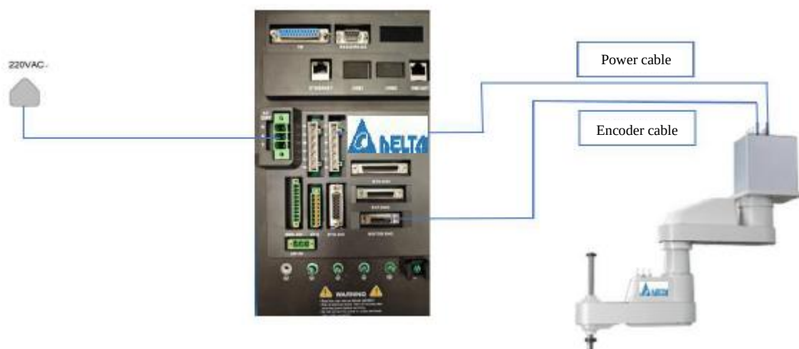
Figure 4-3 Encoder/Power cable connection diagram of Python550F-D6
