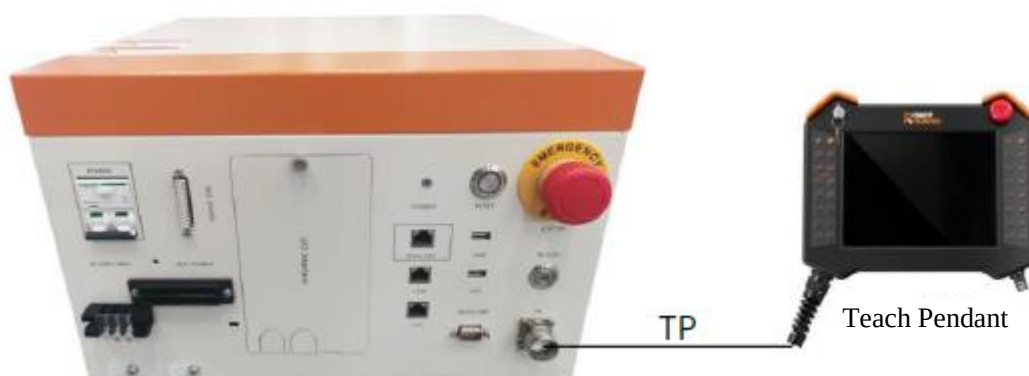
Figure 4-5 Teach Pendant connection diagram
