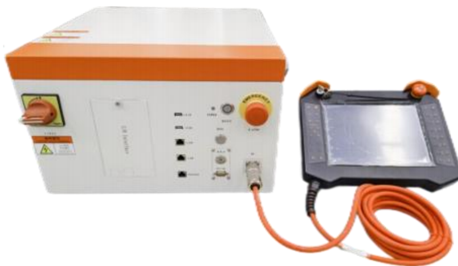
Figure 4-3 Teach Pendant connection diagram
